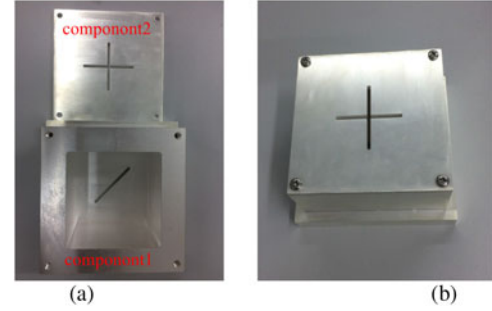
Fig. 7. Photographs of the fabricated CP cavity-backed slot antenna A. (a) Inner view. (b) Outside view.
